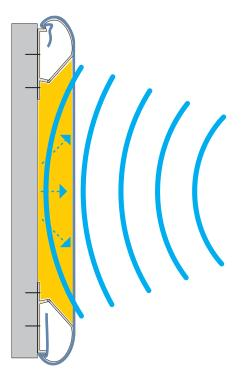
Sound travels through the panel, hits the wall surface and on its journey to and back, is absorbed in the acoustical substrate and dissipated as heat energy.
